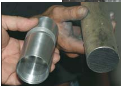
Above: A part on the multi-tasking Doosan Infracore Puma MX 2500 which has just been machined from the raw metal bars seen in the image on the left.
