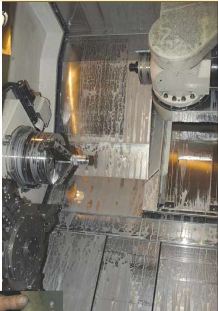
Above: A part on the multi-tasking Doosan Infracore Puma MX 2500 which has just been machined from the raw metal bars seen in the image on the left.
